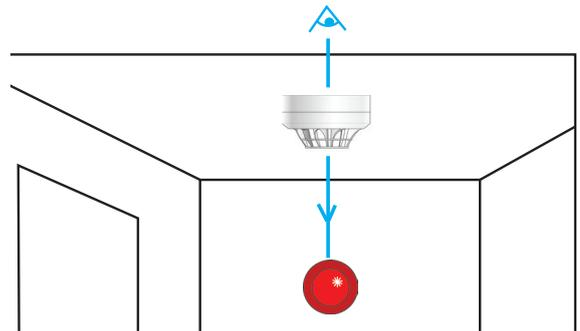
**Figure 8: Example of Using the Line-of-Sight Technique**
